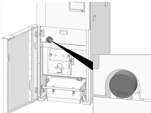
Abb. 2-59\_Position des Manometers
