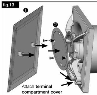
1. Align terminal compartment cover ② with groove, attach and screw to casing.
