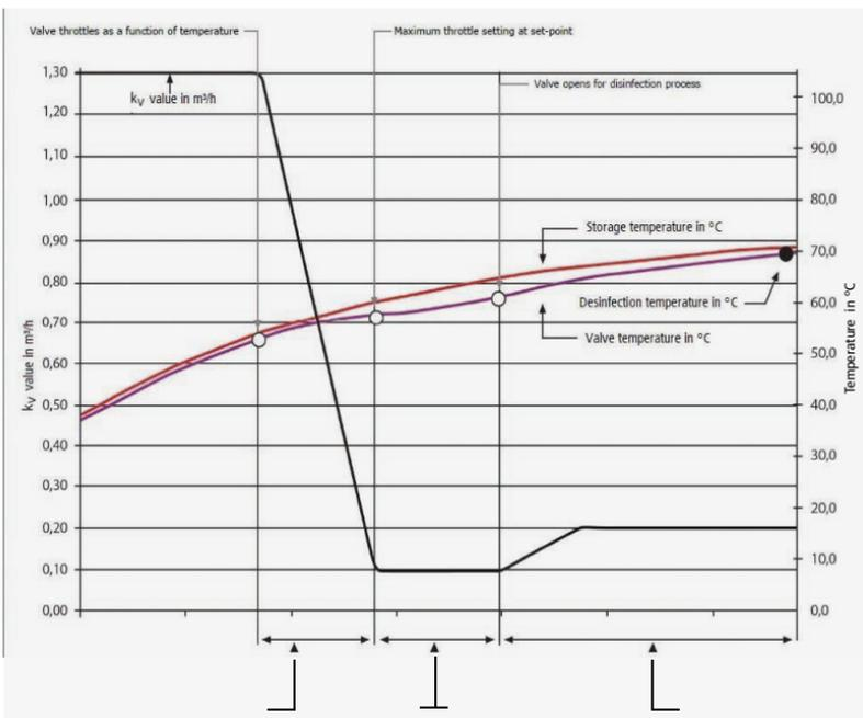
Between 53 °C and set-point 58 °C, the throttling positions are set as a function of temperature.
